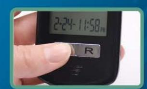
In seconds the meter will audibly say your results as well as display it on the screen. Remove test strip to turn meter off.
