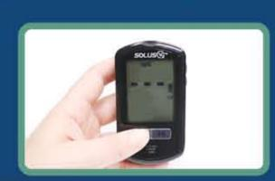
Access Setting Mode: After inserting batteries, press and hold left function button until the meter says "you are now in setting mode".
