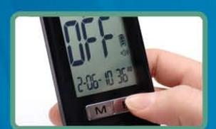
Once all settings have been set and the meter is off, "OFF" will be displayed on the screen along with the month, day, time, battery life, and unit of measure
