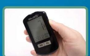
When the meter is off the up/down buttons on the right side of the meter will change the volume. The small round button just below the up/down buttons will change the meter's language if pressed twice.
