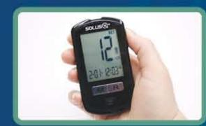
Change Settings: Once in setting mode, the year will be flashing on the screen. Press the up/down buttons on the right side of the meter to change to the year.
