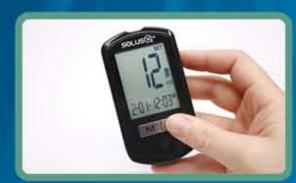
Once the current year is flashing on the screen press the right function button to move to the next setting. Use the up/down buttons on the right side of the meter to change the setting. Repeat this process until all settings are set.
