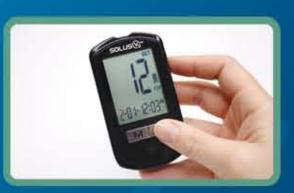
To recall the memory averages press the right function button. Continue to press the button to cycle through 7, 14, 28, 60, and 90 day averages
